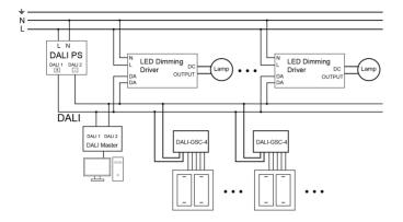
Remark: DALI-200 only provides DALI control signal. You need to use with DALI-130 to increase power supply capacity.
