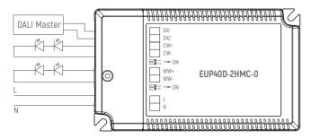
Note: When the DALI signal is not connected, the output power of WW (warm light) channel is full, while that of CW (cold light) channel is not.
