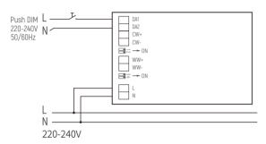
Remark: Only use open push button without indicator light. Maximum cable length between each Unit: 20 meters.
