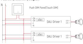
Remark: Only use open push button without indicator light. Maximum cable length between each Unit: 20 meters.
