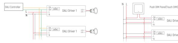
Remark: Only use open push button without indicator light. Maximum cable length between each Unit: 20 meters.
