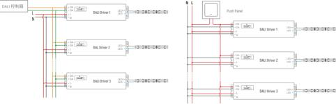
Remark: Only use open push button without indicator light. Maximum cable length between each Unit: 20 meters.
