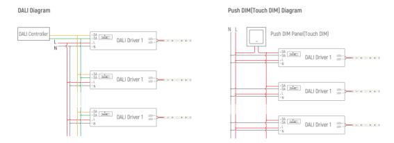
Remark: Only use open push button without indicator light. Maximum cable length between each Unit: 20 meters.
