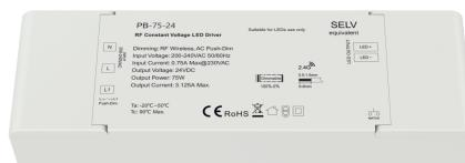
*Dimming interface: RF Wireless, AC Push-Dim. Match with RF 2.4G single color remote control, one RF LED driver accepts up to 10 remote controls. Universal AC input / Full range. 1 channel constant voltage output, Max. total output power 40W. Auto-transmitting function: LED driver automatically transmit signal to another LED driver with 30m control distance. Synchronize on multiple number of LED drivers. Light on/off fade time 3s selectable.*
