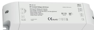
Dimming interface: RF Wireless, AC Push-Dim. Match with RF 2.4G single color remote control, one RF LED driver accepts up to 10 remote controls. Universal AC input / Full range. 1 channel constant voltage output, Max. total output power 40W. Auto-transmitting function: LED driver automatically transmit signal to another LED driver with 30m control distance. Synchronize on multiple number of LED drivers. Light on/off fade time 3s selectable.
