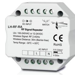
Apply for wireless signal extension, greatly ensures RF communication stability and wide controlling area. Apply for area synchronous dimming to increase synchronous dimming stability. Powered by AC100-240V or DC12-24V. Compatibility with RF 2.4G remote control or panel. Easy to be placed in standard wall junction box.
